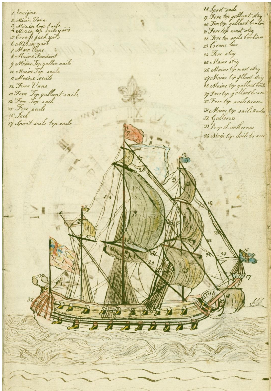
William Woodforde's sketch of a fully rigged warship, with a key to its various components New College Archives, Oxford, NCA 9544
